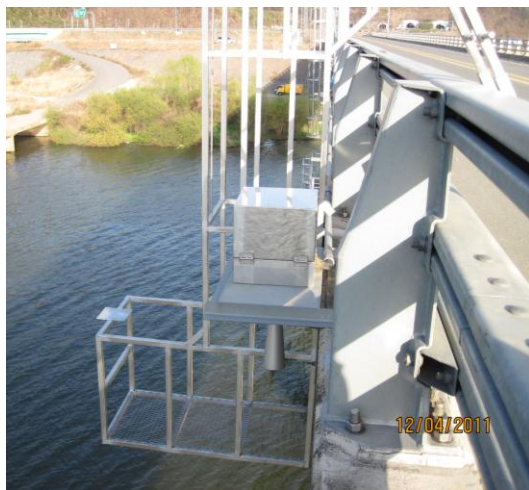
Fig. 4-4 Radar gauge and schematic features
